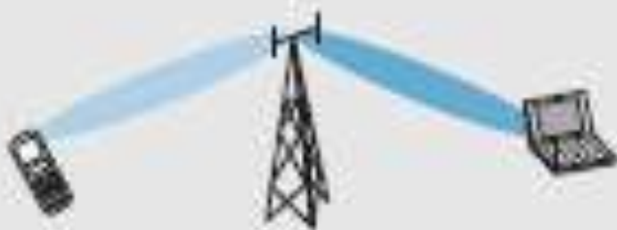
Spatial-division multiple access ("MU-MIMO") for improved capacity (more users per cell)
